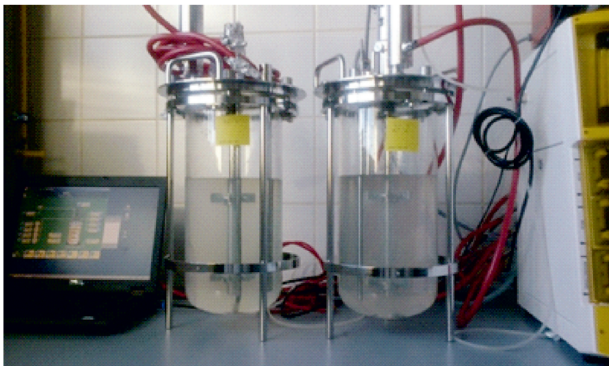
Fig. 3. Bioreactors used for MBC culture on NMS medium (photo by Wolińska A., 2014)
