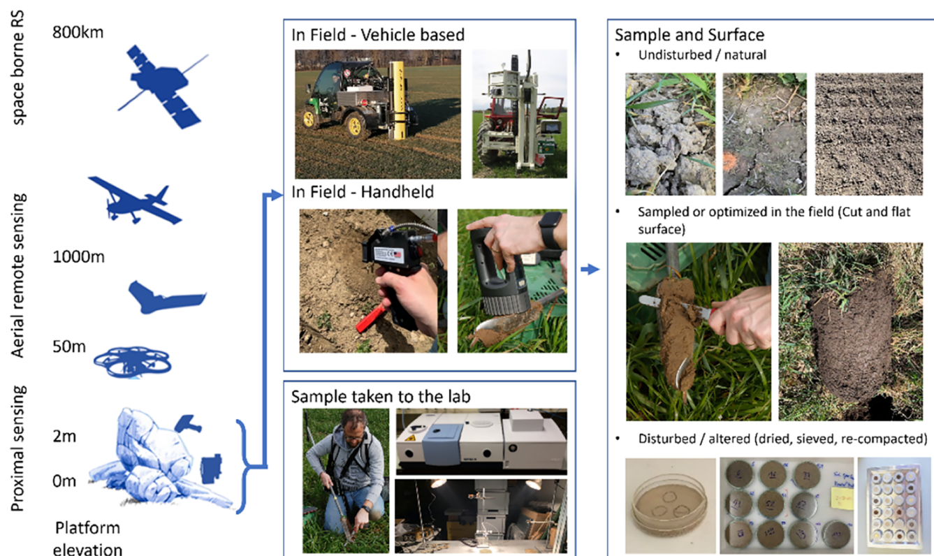
FIGURE 1 Overview of proximal soil sensing as distinguished from remote sensing (left) and a close-up of sensing methodologies used in the field and lab (middle), and examples of surface sample preparation (right). Symbols from Booyesen et al. (2019).
